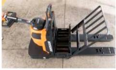
Battery Roller System is Standard Saves time and effort during battery
