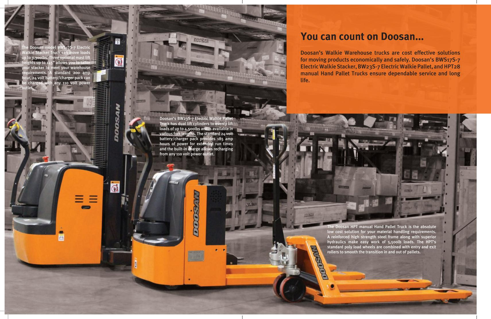
The Doosan Electric Walkie Warehouse Series has AC drive for higher efficiency and lower maintenance costs. Curtis controllers provide reliable performance, smooth acceleration, and seamless directional changes for safer operation. A combo hour meter/battery discharge indicator is standard to track operating hours and reserve power.
