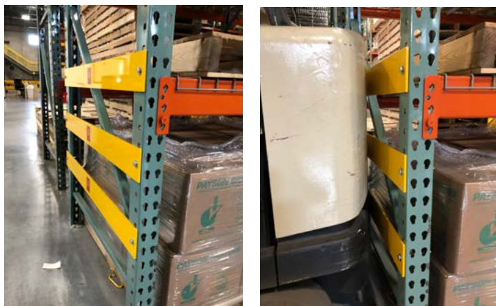
Reinforces rack and protects from impact
