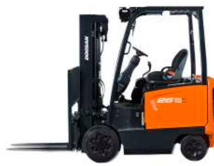
BC20S/BC25S/BC30S/ BC32S-7, BC25SE-7 4,000/5,000/6,000/6,500 lb. Capacity 4-Wheel Cushion Tire Electric, 36/48V
