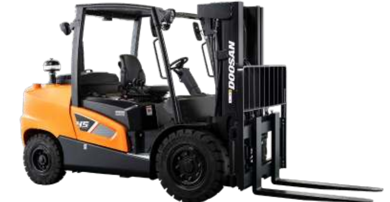
D35S/D40S/D45S, D50C/D55C-9 8,000/9,000/10,000; 11,000/12,000 lb. Cap. Pneumatic Tire IC (Diesel)
