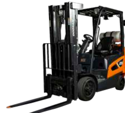
GC20S/GC25S/GC30S/GC33S-9 4,000/5,000/6,000/6,500 lb. Capacity Cushion Tire IC (LP)
