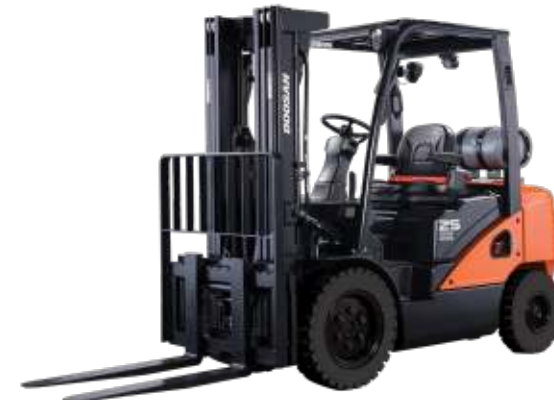
G20N/G25N/G30N/G33N/G35NC-7 G20E/G25E/G30E/G33E/FG35EC-7 4,000/5,000/6,000/6,500/7,000 lb. Capacity Pneumatic Tire IC (LP/DF)
