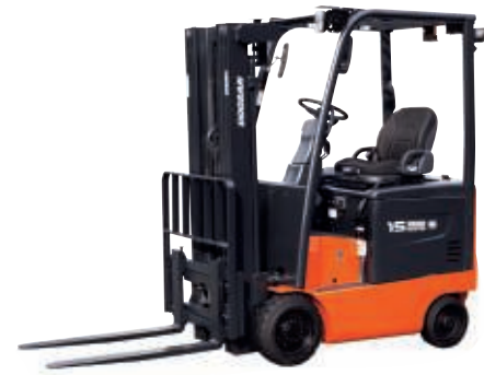
BC15S/BC18S-5, BC20SC-5 3,000/3,500/4,000 lb. Capacity Cushion Tire Electric, 36/48V
