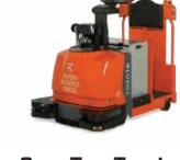
**Core Tow Tractor Automated Forklift** 10,000 lbs.
