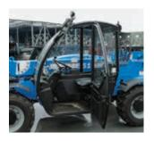
Fully Enclosed Cab Increase operator comfort and decrease fatigue in a clean, dry, quiet cab with standard windshield washer, as well as a heater and defroster for cold climates. Front window doubles as an emergency exit. Left and rear windows open for ventilation. Air conditioning is also available as an option.
